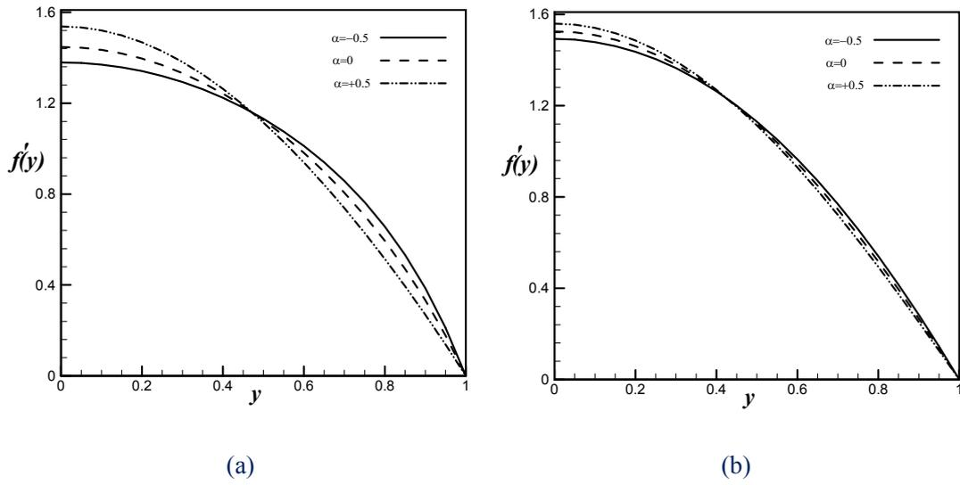
**Fig. 3.**  $f'(y)$  changes shown over a range of  $\alpha$  at (a)  $Re = -5$  (b)  $Re = 5$
